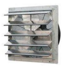
Powered wall vent. This is a workhorse for exhaustion. It would be typical in a shed that you are doing a lot of painting or craft work that has fumes. Also for a cigar shed where you need to exhaust smoke out of the shed. Just remember that if you have to exhaust a lot of air you need to have a supply of good fresh air coming into the shed to displace the bad air.
